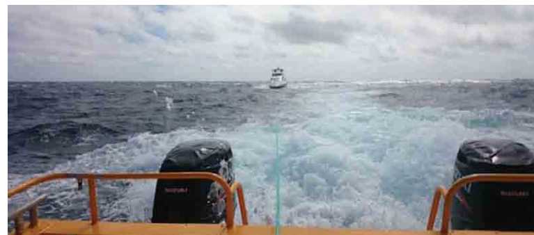
The 250hp Suzukis never missed a beat and made 6kts in the moderate and rough seas.
